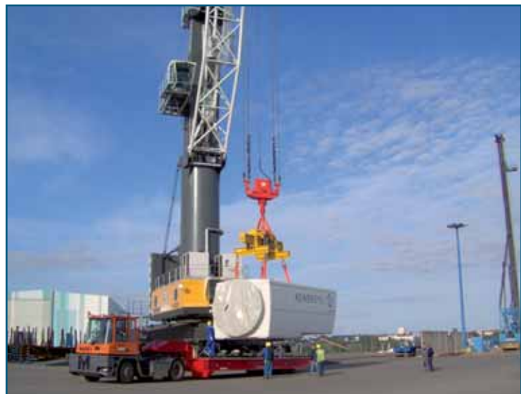
Loading of segments for wind power plants with port equipment
